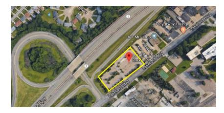
The Wickliffe Park-n-Ride was constructed in 1999. The current layout of the lot is not ADA compliant when three buses are laying over at the same time; as well as, the lot needs to be reconfigured to allow for the bus to approach the electric charging station.
