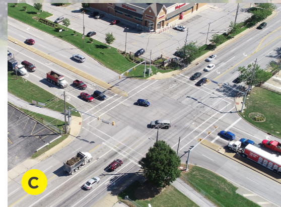
The Vine St/SOM Center Rd intersection is the widest area of the corridor with two driving lanes in each direction, a right turning lane and a left turning lane.
